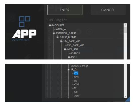
**Note** – In the example shown, [EXTERIOR\_PAINT/ PAINT\_BLEND/ UM\_BASE\_400/ MTR\_400, DC1/ SP\_D/ CV] has been selected
